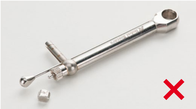
Direction indicator broken
