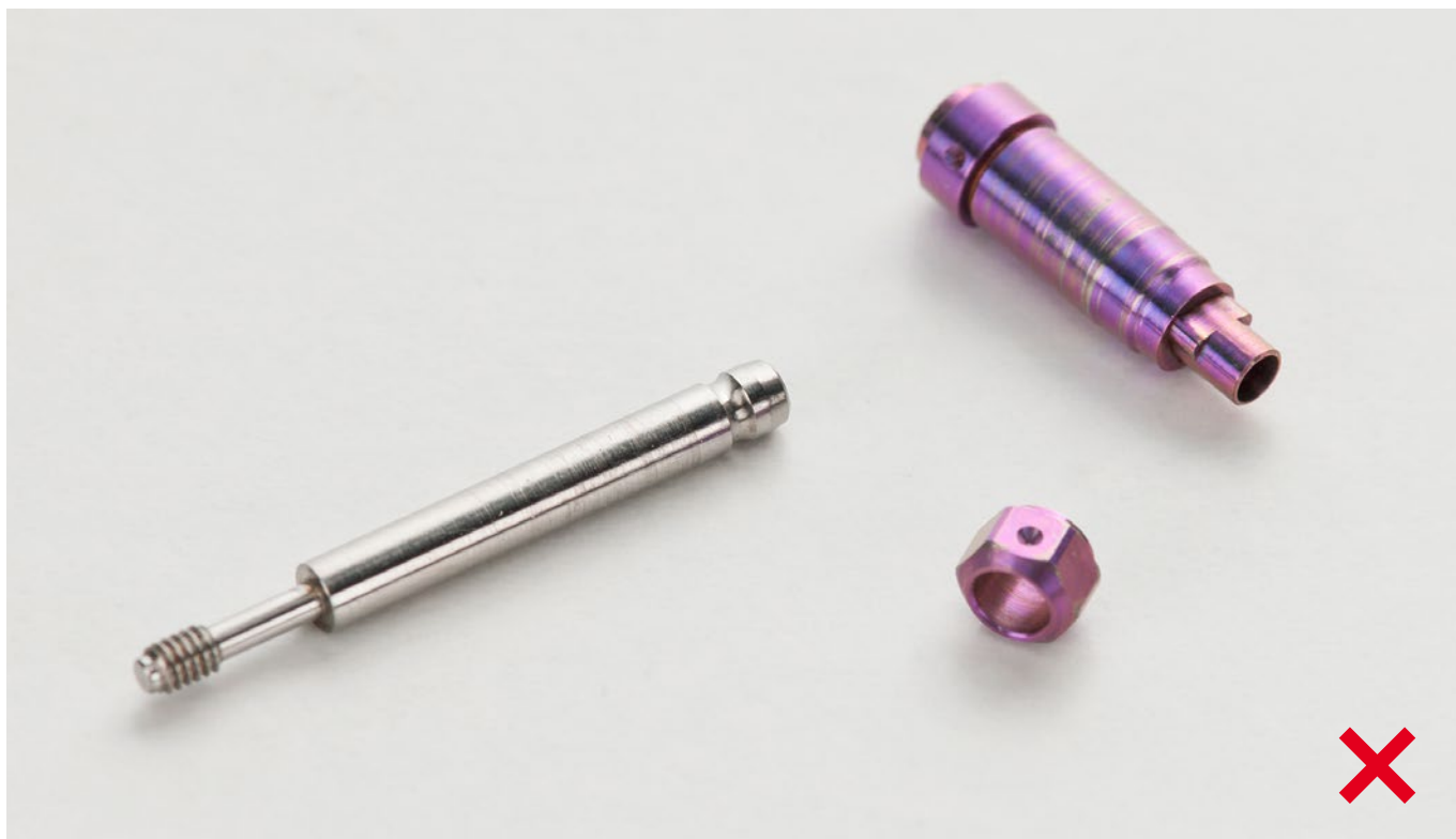
Broken guided implant mount
