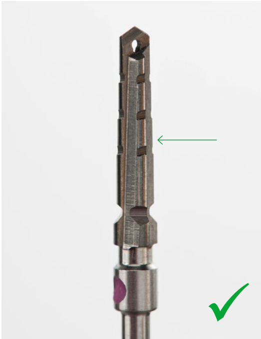
New drill with sharp cutting edges
