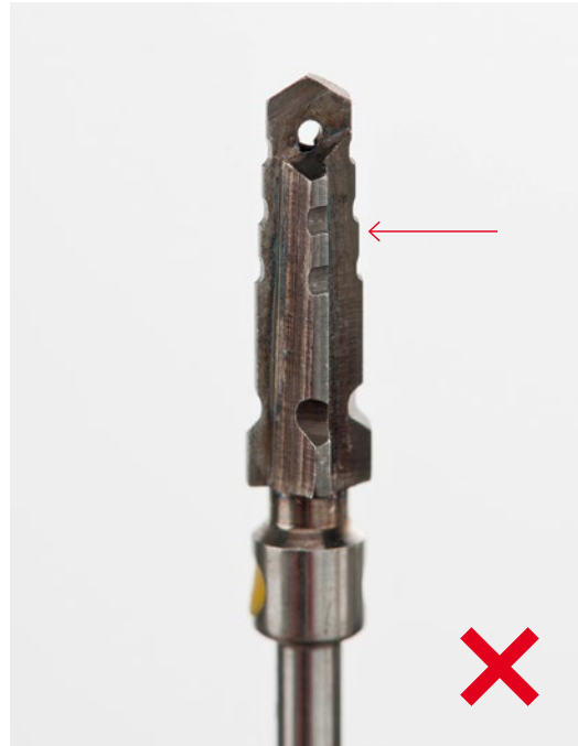
Cutting edges are dull / worn out
