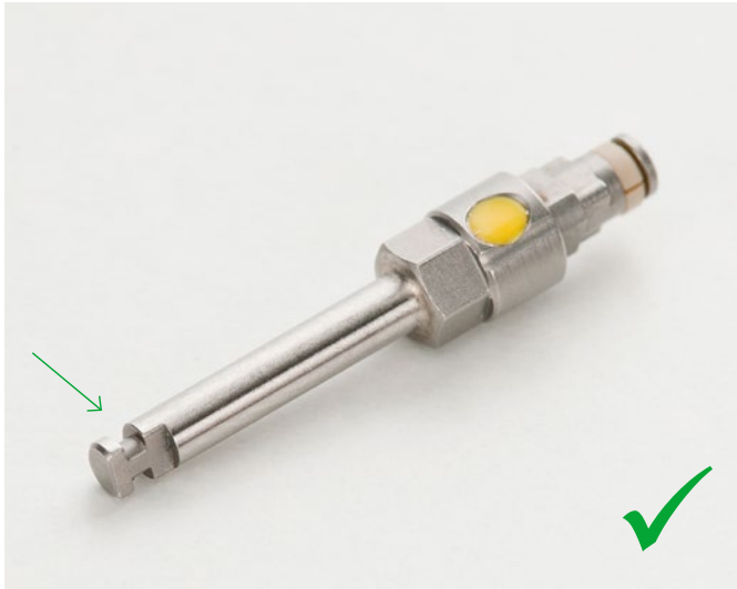
Intact connection to the handpiece
