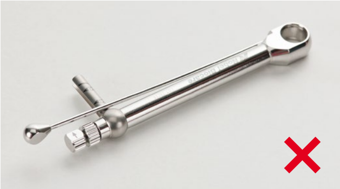
Spring out of guidance pillar
