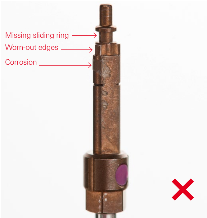
Worn-out implant driver
