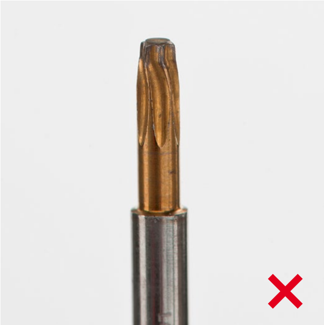
Deformed and worn-out tip
