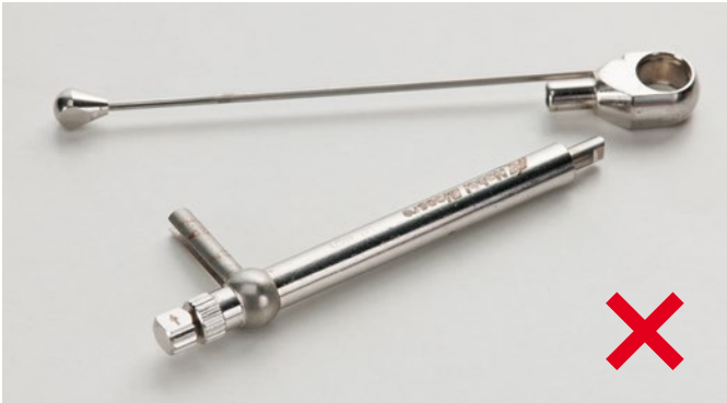
Head of tool broken
