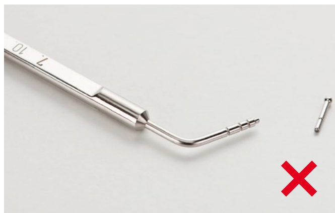
Broken depth probe
