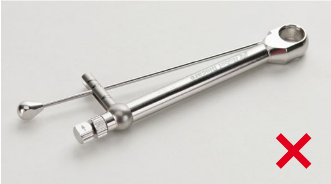
Spring bent due to overload
