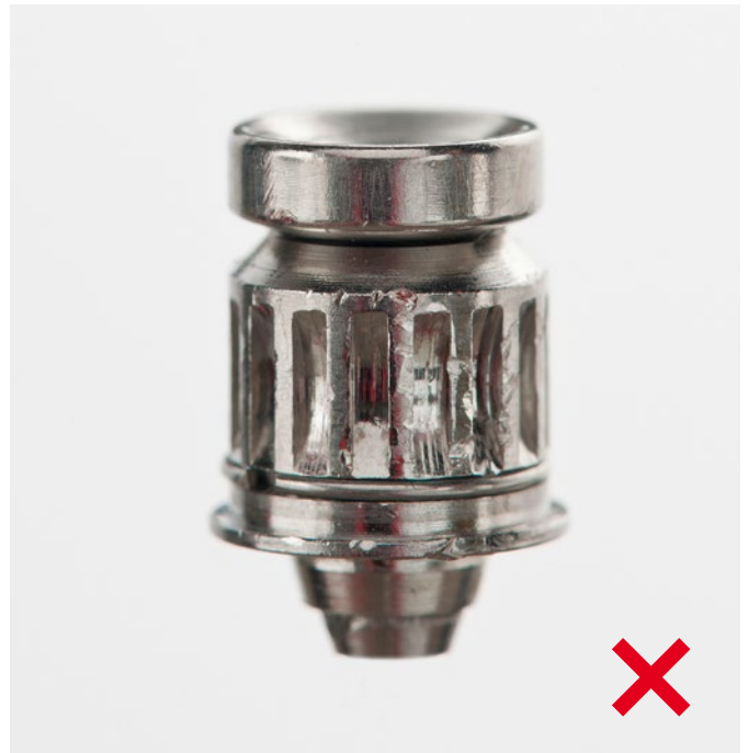
Adapter structure worn out
