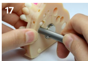
Rotate the Pliers clockwise until the Insertion Screw is fully screwed. The torque applied to the Insertion Screw must not exceed 5 Ncm. (Screw lightly.)
