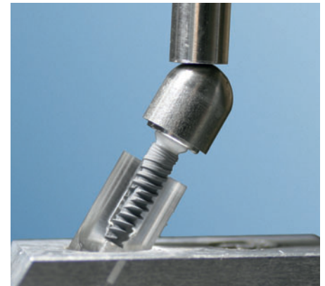
Figure 2: NobelActive NP fatigue testing
