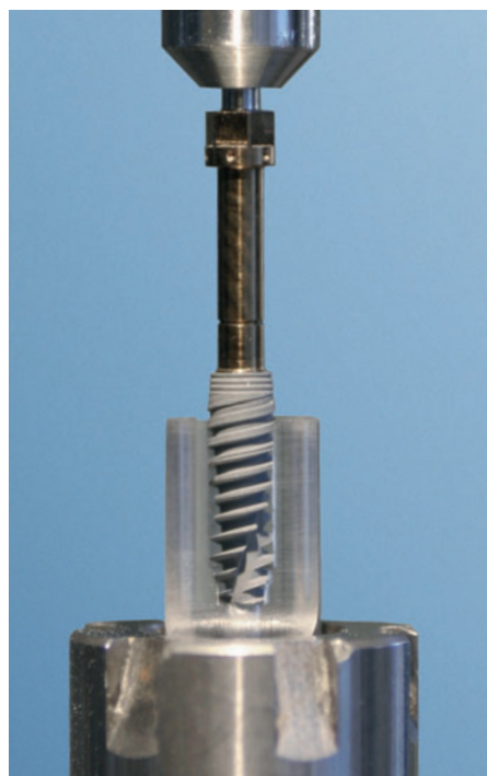
Figure 3: Torque strength testing
